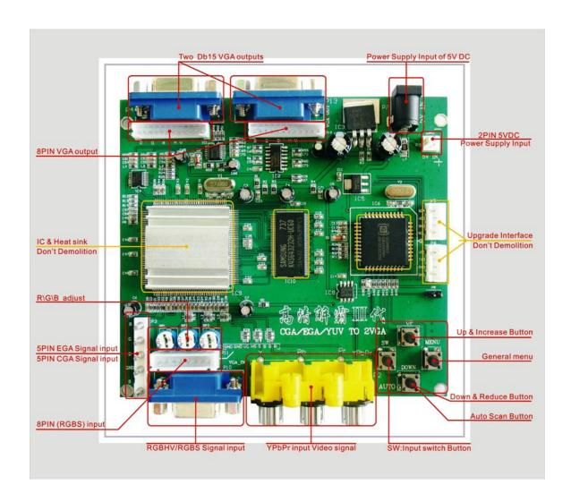
The AT 3800 can easily convert any CGA or EGA input signal to a VGA output signal suitable for display on an LCD monitor of any size.
